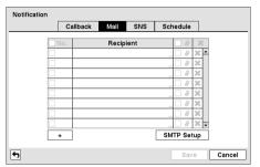
The DVR can be set up to send an email when an event occurs. The Mail account can be turned On or Off by highlighting the boxes under the No. heading and pressing the ⊚ button.
