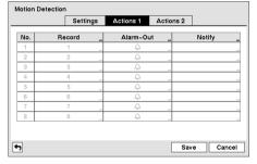
The DVR can be set to react to motion detection differently for each camera. Each camera can be associated with another camera, trigger an Alarm-Out connector, sound the DVR's internal buzzer, notify a number of different devices, and/or move PTZ cameras to preset positions.
