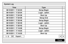
The System Log screen lists system activities (up to 5,000 from the latest) that have occurred along with the time and date. The Haicon will be displayed in the last column for system activities of the remote site. You can scroll through the log pages by using the Up and Down arrows, or you can go directly to a log page by entering the log page number in the box at the bottom left of the screen. Highlight Close and press the 50 button to exit the screen.
