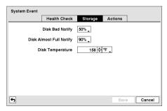
Highlight the box beside Disk Bad Notify, and press the button. Select percentage level of bad disk sectors at which you want the DVR to trigger an alert. Percentage levels range from 10% to 90%.
