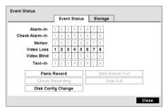
The Event Status screen displays the status of the DVR's systems and inputs. Events will be highlighted, and related channels or events will flicker for five seconds when detected.
