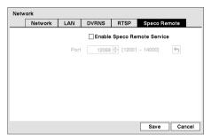
Highlight Enable Speco Remote Service and press the ⊚ button to toggle between On and Off. See *Appendix – Speco Remote* for detailed descriptions of the Speco Remote service.
