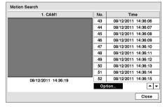
The Motion Search... can be selected from the Search menu while the DVR displays the camera full screen. The Motion Search screen displays a list of motion events. Use the arrow buttons to highlight the event for which you would like to see video and press the (a) (Play/Pause) button to display the video associated with the selected event on the small search screen.
