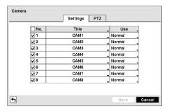
You can turn the camera number On or Off, and you can change the Title of each camera using the virtual keyboard. You can also determine which cameras will display on the monitors by selecting Normal, Covert 1 or Covert 2 from a drop-down list in the Use column.
