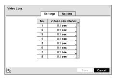
Highlighting the box under the Video Loss Interval heading allows you to set the duration of a signal loss before the DVR will report a Video Loss. The DVR will not consider any signal loss from a camera to be a Video Loss if the detected signal loss is shorter than the interval set on this screen.
