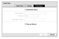
Highlight the box beside Automatic Sync. and press the ⊚ button. This toggles between On and Off.
