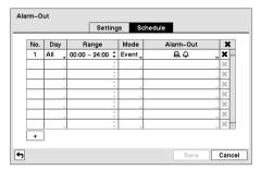
You can add and edit alarm output schedules on this screen. Highlight the + and press the button to add a schedule. Highlighting the boxes under the Column heading and pressing the button allows you to edit the information in those boxes.
