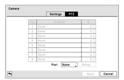
NOTE: You will only be able to set up PTZ devices if the PTZ port is set to RS232 or RS485.
