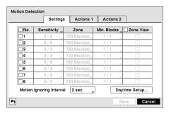
Your DVR has built-in video motion detection. Video motion detection can be turned On or Off for each camera.
