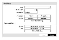
In the Information screen, you can name the site location, assign a System ID number, select the language the screens are displayed in, display software version number, upgrade the software, show the System Log, display recorded time data, and clear all data.
