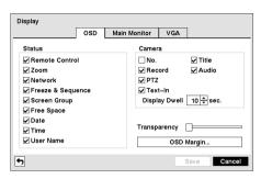
Highlighting an item and pressing the button toggles that item On and Off. When an item is On, there is a checkmark in the box beside it. The following items can be turned On or Off:
