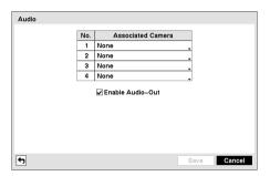
The DVR can record up to four audio inputs. Highlight the box beside the input and press the button. A list of cameras appears, and you can select which camera you want associated with that audio input.
