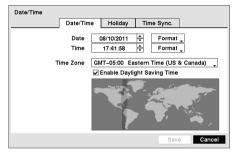
date will highlight. Use the Up and Down arrow buttons to change the number. Use the Left and Right arrow buttons to move between month, date and year. Once you have the correct date, press the 60 button.
