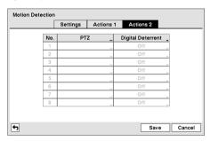
Highlight the desired box under the PTZ heading, and press the  $\odot$  button. A list of PTZ presets appear. Select the preset position for each PTZ camera, where you want PTZ cameras to move to whenever the DVR detects motion on the selected camera's input.
