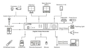
Figure 1 — Typical DVR installation.
