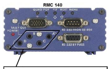
Connect the TD-2 to the RMC 140 Tally Light Output 3.5mm Jack Sockets, via the CB-1 cable.
