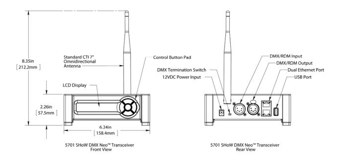
Figure 2, the 5701 SHoW DMX Neo Transceiver
