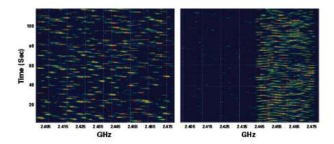
In these Wi-Spy screen shots, the effect of limiting the SHoW DMX bandwidth to WiFi bands 7-12 is clearly shown. In the right hand screen, the portion of the spectrum below 2.466GHz is nearly devoid of activity.
