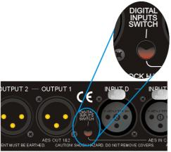
Input selection is via a recessed switch on the rear panel of the unit, between input D and output I. A red LED inside this aperture illuminates to show that the AES digital inputs have been selected.
