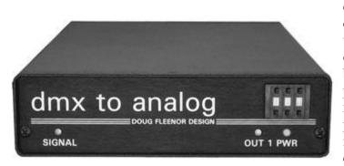
The *DMX to Analog Converter* decodes consecutive DMX512 channels to 0 to 10 volt output. Two versions are available: 24 and 96 output. The starting address is selected by an easy to read (and set) three digit push-wheel switch. The switch is mounted on the front panel along with power, signal, and output 1 mimic indicators. The DMX in and through connectors and the female DB-25 output connector(s) are located on the back panel.
