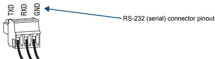
FIG. 34 Wire RS-232 ports for serial data transfer
