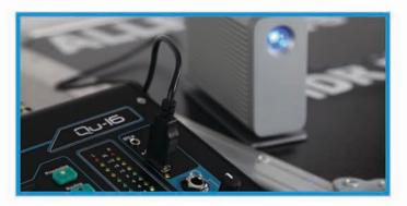
An independent set of controls is provided for quick stereo recording of the main LR or other mix outputs, and a 2-track USB return can be routed to ST3 for playback of stereo WAV files such as walk-in music.
