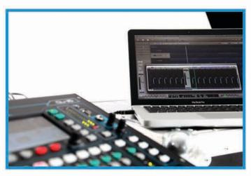
The returns from the Mac can be assigned to the Input channels. The interface is class-compliant on Mac OS X – which means it's truly plug 'n play, with no need to install a driver. It will be recognized straightaway by any DAW supporting Core Audio, including Logic, Cubase, Reaper, and Pro Tools.
