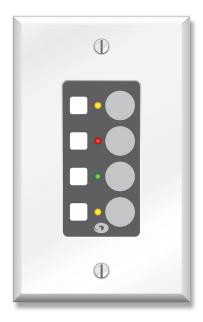
The ARC-SW4e is a modular remote control wall panel with four switches that are programmable as momentary, latched or radio buttons. ARC-SW4e provides simple control over mutes, source selection and preset triggering. Corresponding tri-color LEDs provide user feedback. LEDs may be linked to buttons, or, LEDs and buttons may be programmed independently. Symetrix DSP software performs all control assignments, including button and LED functionality, parameter limits and firmware version upgrades.
