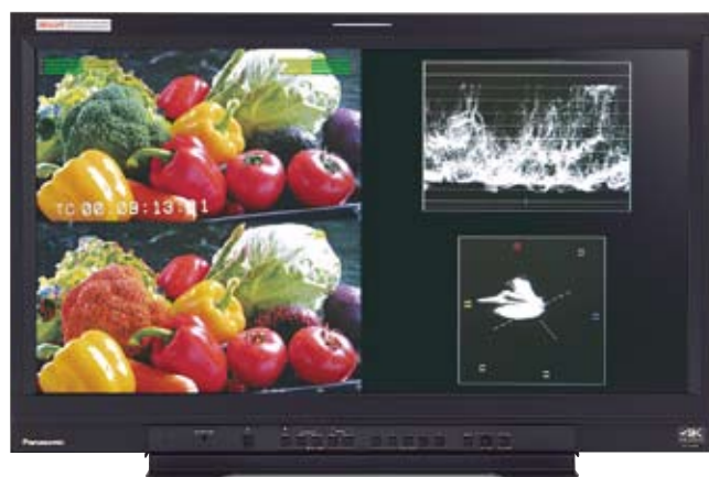
Sample display of the input source image (upper left), Focus-in-Red (lower left), WFM (upper right) and VSC (lower right) (All images are simulated.)
