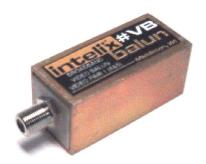
The Intelix VB Balun transmits broadband video signals via Cat 5 unshielded twisted pair (UTP) cable. Used in pairs, the VB transmits 120+ channels (850 MHz) in CATV spectrum and is ideal for cable TV distribution and media retrieval systems.
