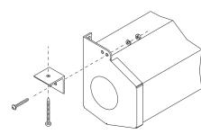
Use the **front** mounting hole in the endcap for recessed mounting flush with the ceiling. Attach angle (not included) to screen then position and properly anchor screw fasteners (not included) into ceiling joists or other solid surface. Recommended hardware: For mounting into wood or ceiling joist, use <sup>3</sup>/<sub>16</sub>" bolts.
