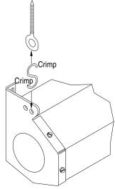
Use the holes at the **front** of the mounting bracket for suspended mounting. Position and properly anchor screw eyes or other fasteners (not included) into ceiling joists or other solid surface. Suspend "S" hooks (not included) from fasteners and hook through **front** mounting hole in the endcap. For added safety, crimp both ends of the "S" hooks so the screen cannot come off.
