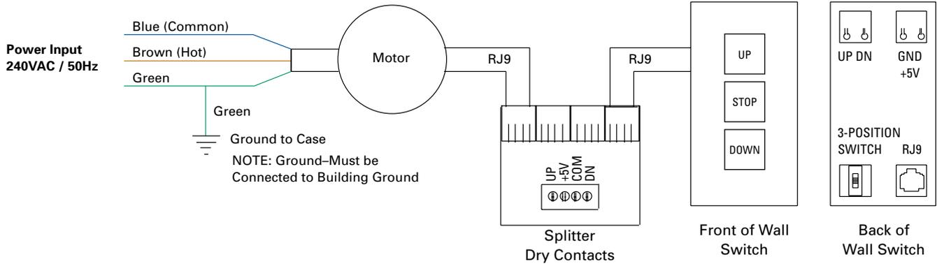
**240V WIRING DIAGRAM WITH OPTIONAL BUILT-IN VIDEO PROJECTOR INTERFACE**
