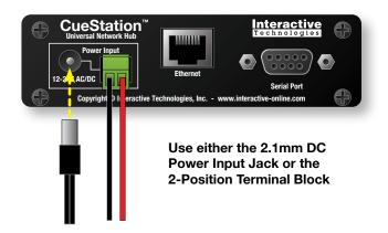
There are two power input jacks on the Hub, a 2.1mm DC Input Jack and a 2-Position Terminal Block. You can use either one, but not both. If the 2.1mm DC Input Jack is used, it electrically disconnects the circuit from the Terminal Block input.
