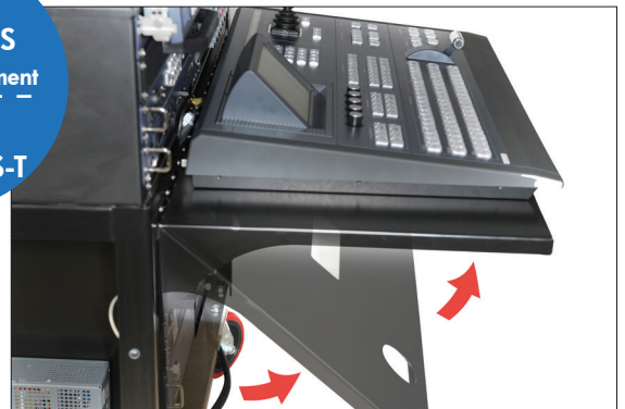
The control panel is folded down for transport. When unfolded, it functions as the tray holder for the SE-3000 keyboard.
