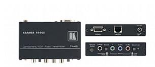
The TP-45 is a twisted pair transmitter for component video (YUV) or computer graphics video and unbalanced stereo audio or S/PDIF audio signals. The TP-45 transmitter converts audio and video to a twisted pair signal and the TP-46 converts the twisted pair signal back into audio and video signals.
