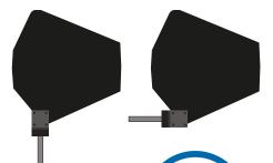
The mounting block can be rotated to allow horizontal or vertical mounting
