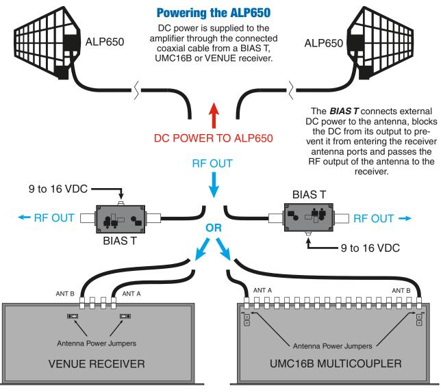
The **VENUE** receiver also includes a DC power pass-through to operate the ALP650 antenna amplifier. Jumpers on the circuit board enable and disable the DC power.
