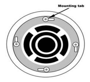
Be sure to position the four Mounting Tabs on your OWI speaker inward then insert the four (4) screws (supplied) from the front of the speaker into the screw opening.
