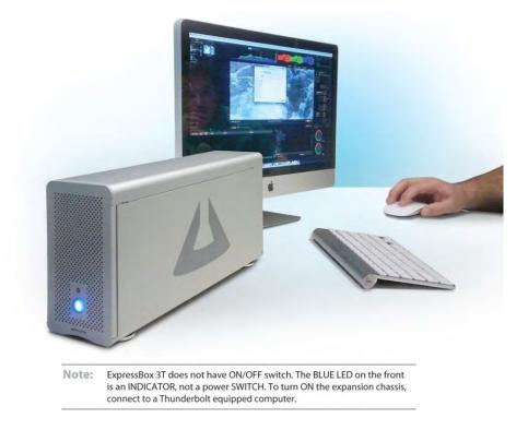
The Blue light on the front of ExpressBox 3T is not an on off push button, it simply indicates whether the chassis is on or off.
