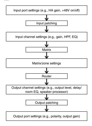
As necessary, make input patching and output patching settings to specify the audio signal flow of the devices connected to the MTX3's [INPUT] /[ST IN]/[OUTPUT]/ [YDIF] connectors.
