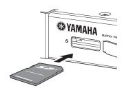
When the SD memory card has been correctly recognized, the [SD/ACT] indicator (page 8) will light. The [SD/ACT] indicator will blink while the card is being accessed.
