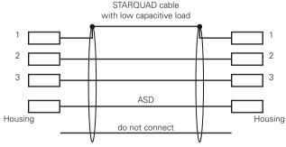
Capacity between ASD line to shield total < 2.7nF
