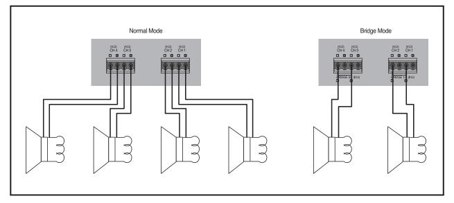
Only connect speakers with an impedance equal to or greater than those specified below.
