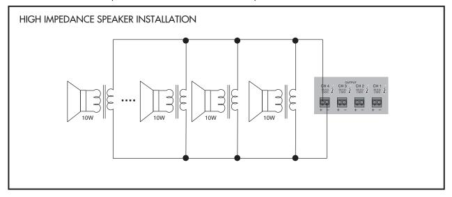
Only connect speakers with an impedance equal to or greater than those specified below.
