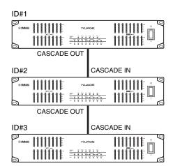
Up to eight devices can be connected in this way.
