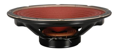
The 8C10PAOT is an 8" O.D. loudspeaker with a 10 oz. magnet, 8 Ohm nominal impedance and a phenolic resin impregnated, moisture resistant cone. Frame has a black powder coat finish.
