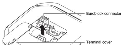
3 After loosening the terminal screws of the Euroblock connector with a flat-blade screwdriver, insert the cable into each terminal and tighten the screws. Make sure that cables cannot be pulled out.
