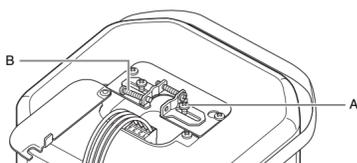
7 Hold the cable in the strain relief clamp, then tighten screws A and B.
