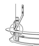
To release the speaker from the O-ring, press the Anti-Drop tabs. These are located above the ▲ mark near the edge of the baffle's face.
