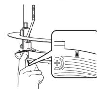
3 Turn the screwdriver a half turn counterclockwise to loosen the attachment screw (located beside the ▲ mark). This makes the clamp easier to align in the channel.
