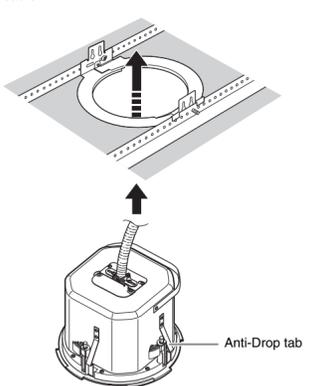
When all the Anti-Drop tabs cross over the O-ring, the speaker is held temporarily.
