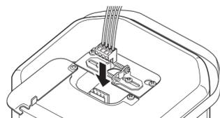
5 Loosen the screw A of the strain relief clamp.
