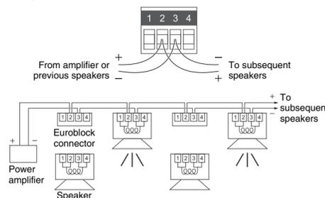
4 Plug the connected Euroblock connector into the socket in the speaker.
