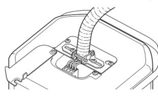
8 Close the terminal cover and tighten the screw.
