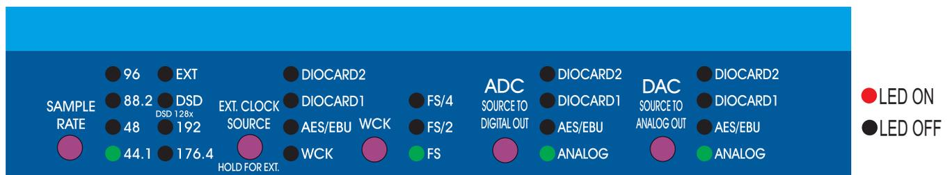
In this mode both the AD and DA run on the internal clock. This mode also provides the lowest jitter and most sonically robust performance. External recorders (such as DAW etc) must be synchronized either to AD digital outputs (any format: AES or DIOCARD1 or DIOCARD2) or to the converter Wordclock output.
