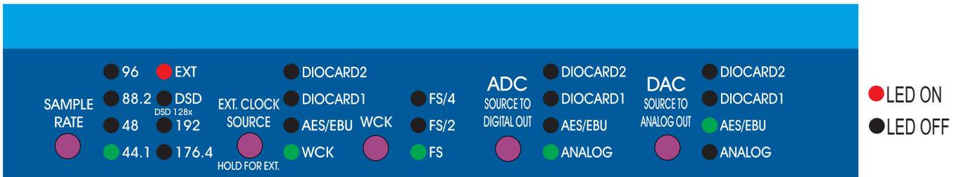
In this mode both the AD and DA run on an external clock. Holding the "Ext. Clock Source" button selects this mode. Although this mode does not provide the lowest jitter performance it might be desirable for systemic reasons. External recorders (such as DAW etc) can be synchronized to external wordclock sources OR AD digital outputs (any format: AES or DIOCARD1 or DIOCARD2) OR to converter Wordclock output.
