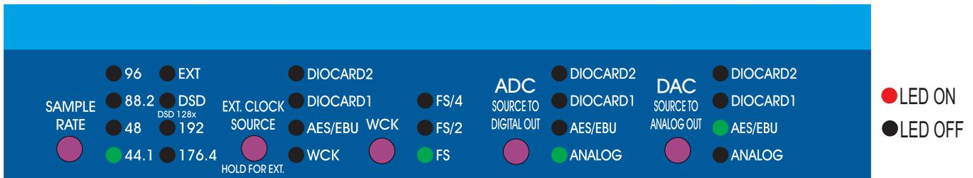
In this mode both the AD and DA run on the internal clock. This mode provides the lowest jitter and most sonically robust performance. External recorders (such as DAW etc) have to be synchronized either to the AD digital outputs (any format: AES or DIOCARD1 or DIOCARD2) or to the converter Wordclock output.
