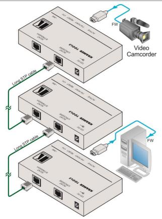
Figure 3: Connecting Three TP-300FW Units to Extend the Distance to 200m
