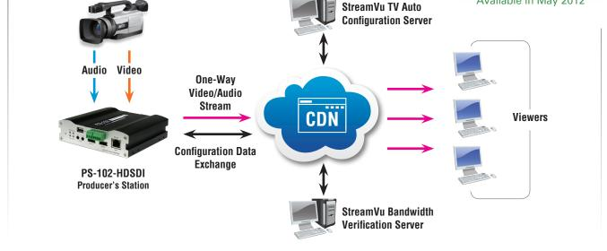
The Producer Station is a self contained appliance that accepts the audio & video feeds of the event to broadcast and processes the feed to IP for transport to the StreamVu TV server via a high speed broadband / Internet connection. The Producer Station contains all hardware, software, audio & video processing and encoding needed for live streaming.
