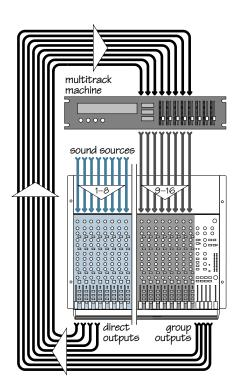
The outputs of the multitrack are then patched to the next eight LINE [2] inputs on the 1604-VLZ3 (multi-track out 1 to LINE input 9, 2 to 10, 3 to 11, etc.). Aha! That's why it says "TRACK 1" next to channel 9's fader, "TRACK 2" next to channel 10, and so forth. These channels (9–16) will be assigned to the mixer's output section, delivering the signals to their ultimate destination, which may be your mixdown 2-track, your control room system, or your headphones.
