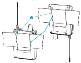
The belt clip is detachable so that you can also attach the diversity receiver with the antenna pointing downwards. To do so, withdraw the belt clip from its fixing points and attach it the other way round. The belt clip is secured so that it cannot slide out of its fixing points accidentally.
