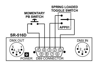
If a SR-516s simple switch functions are set to factory default operation then the switches will operate as follows for the connection example shown above.
