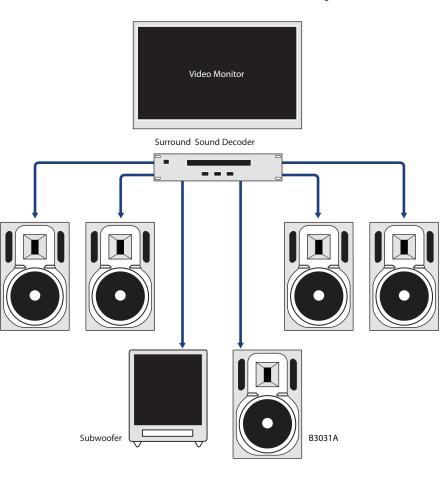
Placement is also critical. Ideally, all loudspeakers should be placed away from walls to ensure proper bass response. But fear not, B3030A/B3031A monitors feature Room Compensation switches so you can place them against walls, or even in corners. Walls tend to enhance low-frequency content, and corners exaggerate bass even more, but your TRUTH monitor can be custom-tailored to provide honest bass response for your situation, with the simple flick of a switch or two.
