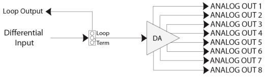
Figure 1. Simplified Block Diagram of the 9231 Functions
