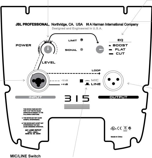
The MIC/ LINE switch affects only the INPUT. It selects between two sensitivity ranges. This switch is used to match the input sensitivity of the FON515 with the output level of the device connected to INPLIT
