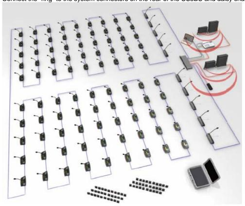
Use no cables that are longer than 330 feet (100 m) to connect one microphone station to another.
