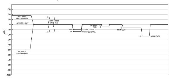
This diagram shows the gain levels in dBu, and the range of adjustment of the signal level as it wanders through the various circuitry inside the mixer. The left side is the input, where the signals enter the mixer, and the right side is the main output.
