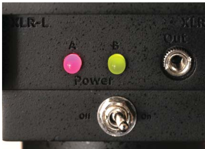
Battery 'A' voltage is low, needs replacement
