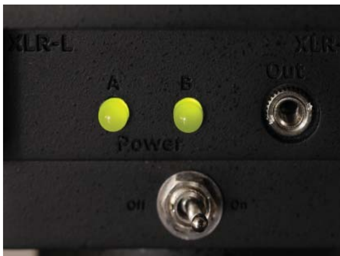
Both batteries are within operating voltage range
