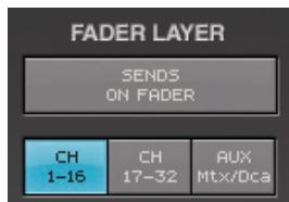
These buttons switch the layer operated by fader modules 1–16. The currently selected layer is shown in blue.
