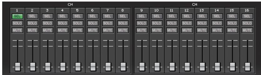
Use these to operate the input channels, AUX, MTX, and DCA.
