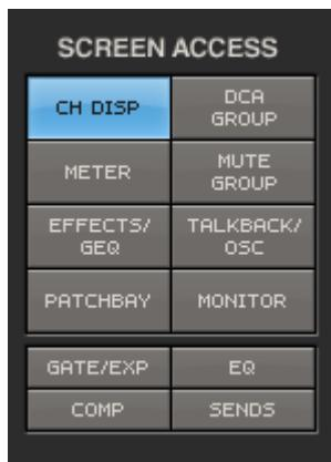
These buttons switch the content of the basic screen area. The button corresponding to the currently shown screen or popup is shown in blue.
