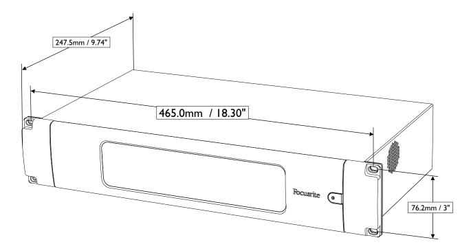
RedNet 1 requires 2U of vertical rackspace and at least 350 mm of rack depth, to allow for cables. RedNet 1 weighs 4.12 kg and for installations in a fixed environment (e.g., a studio), the front panel mounting screws will provide adequate support. If the units are to be used in a mobile situation (e.g., flight-cased for touring, etc.), consideration should be given to using side support rails within the rack.
