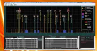
The "one click" and "click and drag" functions make the RF-intermodPro incredibly fast. Once you have your screen set you will see color bars marking harmonics to avoid in setting your wireless devices, and warning icons showing frequencies with interference.
