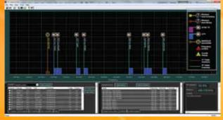
Based on zip-code data the RF-intermodPro<sup>™</sup> automatically selects TV stations, NTSC, DTV and other transmitters as indicators are positioned on the screen showing the frequency locations.
