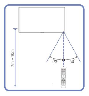
Use the remote control within 7m to 10m from the sensor on the product at an angle of 30° from the left and right.
