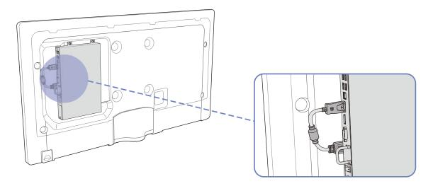
Connect the DP-HDMI cable to the [HDMI IN] port on the product and the [MAGICINFO OUT] port on the network box.
