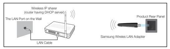
Samsung's Wireless LAN adapter is sold separately and is offered by selected retailers, Ecommerce sites, and Samsungparts.com. Samsung's Wireless LAN adapter supports the IEEE 802.11a/b/g and n communication protocols. Samsung recommends using IEEE 802.11n. When you play video over a network connection, the video may not play smoothly.
