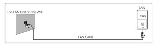
• If you have a Dynamic Network, you should use an ADSL modem or router that supports the Dynamic Host Configuration Protocol (DHCP). Modems and routers that support DHCP automatically provide the IP address, subnet mask, gateway, and DNS values your product needs to
