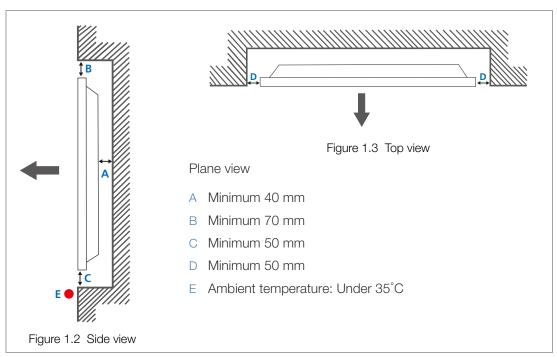
When installing the product on an indented wall, allow at least the space specified above between the product and wall for ventilation and ensure that the ambient temperature is kept below 35°C.
