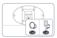
Turn the connecting screw at the bottom of the stand fully so that it is completely fixed.
