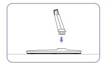
Insert the Stand Connector into the Stand in the direction shown by the figure.
