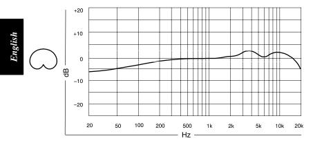
FIGURE 2. TYPICAL FREQUENCY RESPONSE
