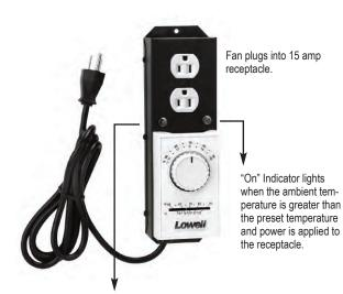
Stand-by Indicator lights when the ambient temperature is below the preset temperature (fan must be connected to the output for indicator to operate).
