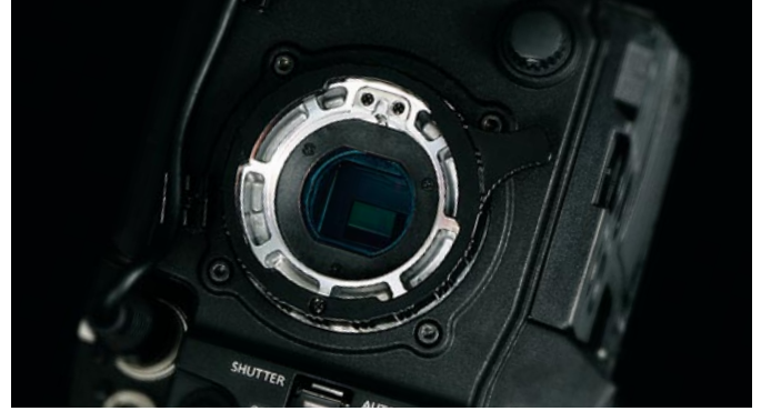
The 2/3-type bayonet mount interchangeable lens system
