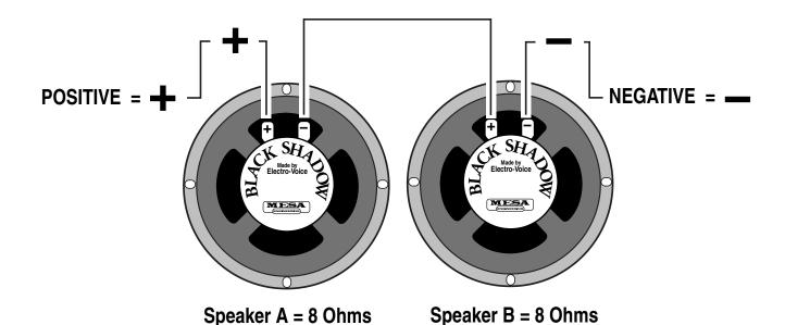
SERIES: Connect the Negative side of Speaker A to the Positive side of Speaker B
