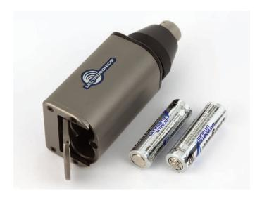
The battery compartment door is hinged to the housing and remains attached to the transmitter when opened. It securely latches in place and applies pressure to the batteries when closed. The two AA batteries are connected in series through a conductive plate on the door.
