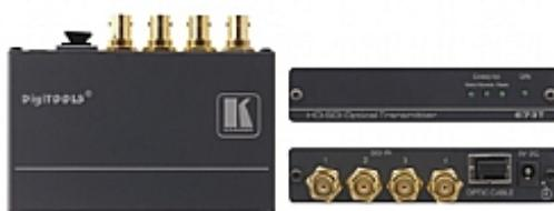
The 673T and 673R are a high-performance fiber optic transmitter and receiver for video signals up to 3G HD-SDI and dual link HD-SDI signals. The 673T converts up to four channels of SDI signals on BNC connectors to an optical signal that is transmitted over a single fiber optic cable. The 673R converts the optical signal back to SDI signals.
