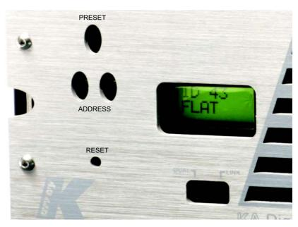
order to remote your system, you need to set each module on a different address, so that, in your chain, no one module will have the same address. Two rotary encoders allow you to set the desired address number that will appear on the top line of the display. Using the remote control software it is possible to mute each system, select a desired preset loaded on-board or download a new preset pack.
