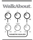
is possible with the only limit being your imagination. As mentioned earlier, the **EQ** is an in-line type, which means that it is in the signal path at all times. If you do not wish to shape your signal with the **EQ** section of the preamp, simply leave all the controls set to 12:00 (straight up) and the **EQ** will pass the signal unaffected. This 12:00 setting would be considered "flat" or in other words, basically bypassed.
