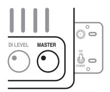
**NOTE:** Use the **MASTER** output level control with care. The **WalkAbouth** is capable of very loud output volumes that could potentially cause damage to your hearing or the hearing of others. May we suggest always beginning your set-up by zeroing-out the **MASTER** output level control to avoid accidental volume attacks on unsuspecting bandmates, engineers or audiences.
