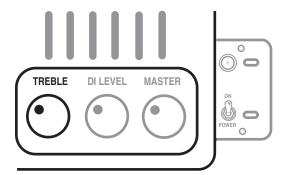
As the control is increased past 12:00, it produces a 6db per octave rise in gain starting at 723Hz until +20db is reached. From this point, gain remains constant at +20db for all frequencies above 723Hz all the way out to 20Khz. This scheme lends a sweetness of sound while retaining all the necessary cut and focus associated with a traditional passive **TREBLE** control.
