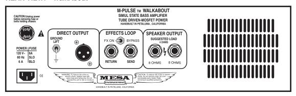
**FUSE:** This is the A.C. Mains Fuse for the *WalkAbout* REPLACE ONLY WITH A SLO-BLO TYPE FUSE OF THE PROPER RATING. THIS IS EXTREMELY IMPORTANT, AS THE *WalkAbout* DRAWS A SUBSTANTIAL AMOUNT OF CURRENT AT HIGH OUTPUT LEVEL SETTINGS.
