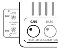
As the **GAIN** control is increased past 12:00 a richer, more "well-rounded" voice becomes dominant and headroom starts to diminish in increments until eventually, a tube overdrive sound appears as the 12AX7 input tube is driven into saturation.
