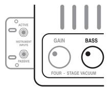
The **BASS** control is actually a gain and frequency control all rolled into one with the Q center at 55Hz and harmonics in both low and high directions are affected because of its broader band nature. As the control is increased past 12:00 there is a 6db per octave rise in gain with the frequency topping out at 321Hz. With 12:00 straight-up representing "flat" (a no boost/no cut setting).
