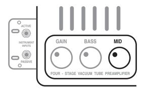
this control is a **boost only**, and while it can competently remove this broad spectrum of midrange from the mix, it cannot provide the extreme attenuation of an active style control.
